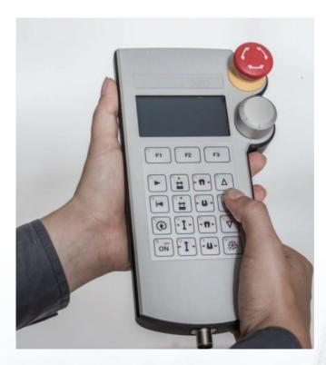
In an emergency case, test can be stopped immediately by pushing the emergency button on the Remote Control console.
